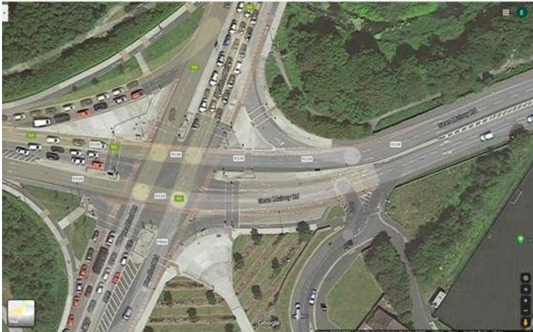
***ABOVE: FIG 3: Intersection at Headford Road junction, Galway City. Note: there is no priority for cyclists; cycle lane suddenly ends forcing cyclist to merge traffic (there is kerb to the footpath) with cars passing at speeds of 50km+. Drains are positioned in such a way that bike trailers can fall in, causing serious danger to children in trailers.***
